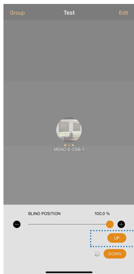
6. Hold the 'UP' button immediately after step 5 and release when the blind has reached the upper limit. The blind is now calibrated.
