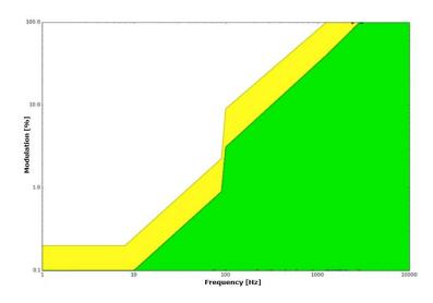
Thanks to its 3,4kHz dimming frequency, the LINE-4CC-CASAMBI effectively reduces the occurrence of the Flicker phenomenon. Depending on an individual's sensitivity and the nature of their activities, flickering can impact one's well-being, even if the changes in luminance are beyond the threshold detectable by the human eye.
