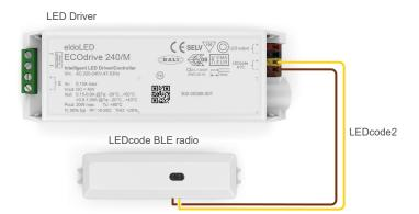
Wiring diagram BT-L2C1
