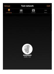
With a single "tap" on the device you can switch it "on" or "off". You can also "tap & hold" the device and then by sliding your finger to left and to the right you can adjust the output of DMR.733 from 0% to 100% accordingly.
