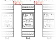
Caution: Leaving no gap/space between the dimmers (for cases 2 & 3) and other components in the rail, might damage the dimmer(s) permanently!
