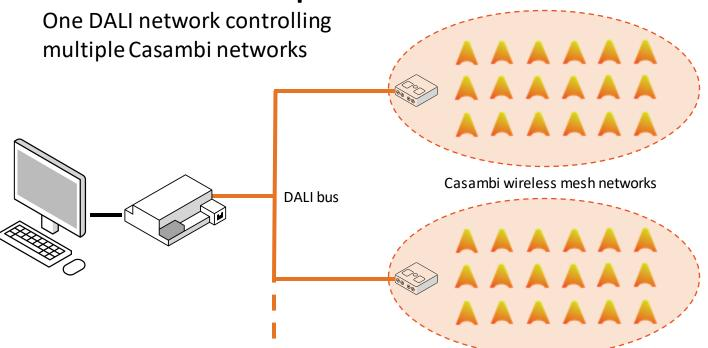
Max. total luminaires + input devices is the same as for one DALI network (CBU-DCS not included)
