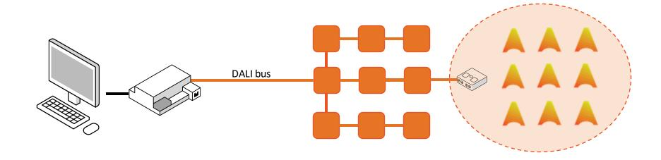
Max. total luminaires + input devices is the same as for one DALI network (CBU-DCS not included)
