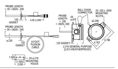
The Series TE Duct and Immersion Building Automation Temperature Sensors can be used to monitor air or water temperature throughout a building management system or an air handler unit. Duct or immersion options available with or without an
