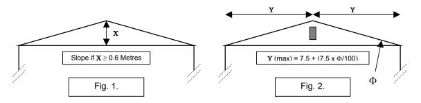
When a Detector is positioned in the apex of a ceiling (See Fig. 2), the lateral beam distance covered (Y) can be increased in relation to the angle of pitch ( $\Phi$ ), up to a maximum of 25%.
