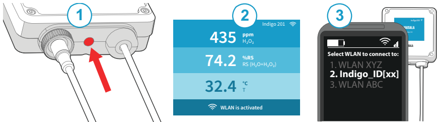
Figure 18 Enabling and accessing wireless configuration interface of Indigo 200
