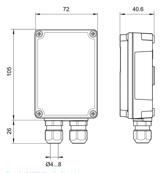
Figure 2 GMP250 Relay Box Dimensions
