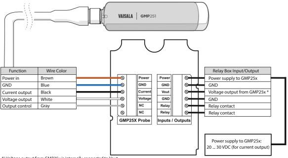
\*) Voltage output from GMP25x is internally connected to  $\overline{\text{Vout}}$
