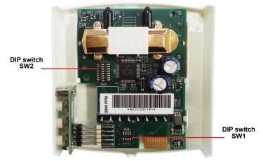
Figure 6: Internal view of transmitter
