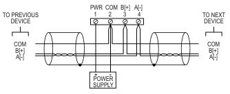
Figure 3: Local power supply wiring
