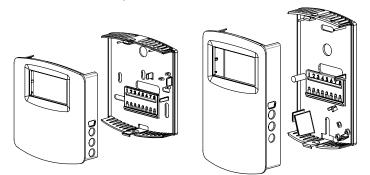
Figure 1: Removal of cover from back plate
