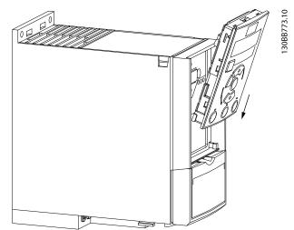
Illustration 1.1 Position the LCP in the Frequency Converter
