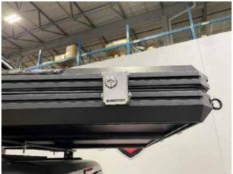
4.) Install ladder brackets using supplied hardware. (Ensure ladder brackets are spaced so the ladder fits onto them). Then install the awning rod supports and shoe bag eyelets.
