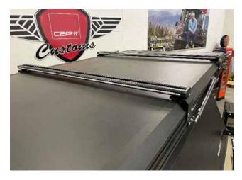
3.) Install two main tent latches, one on each side of the tent using supplied hardware.
