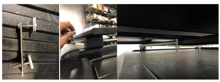
2.) Assemble supplied crossbars on bench and then install on tent using the supplied hardware. (The crossbars have two height settings, see red circles on image below. Set according to the accessories you're mounting on it.) Crossbar spacing on the tent is your choice.
