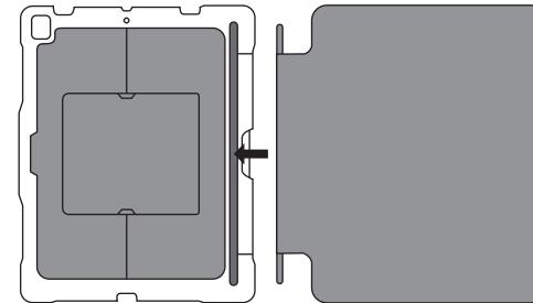
2. Press the connection axis and make sure the connection is stable.
