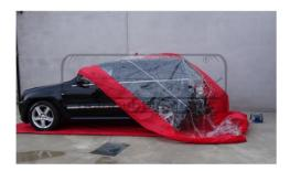
Power up the fan, whilst making sure air can flow freely, observe inflation process for any problems.  Once inflated, check that Bubbles are not rubbing any part of body work. For outdoor products, use top eyelets to stabilise the Bubble from swaying in the wind and rubbing the body.
