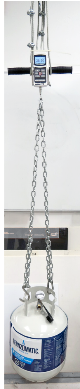
Figure 10: Weighing propane tank
