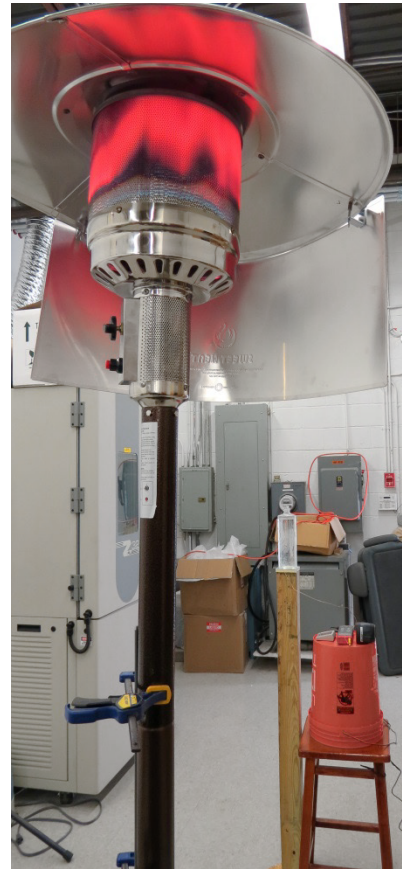
Figure 6: Bottle of water heating directly behind (rear) reflector unit
