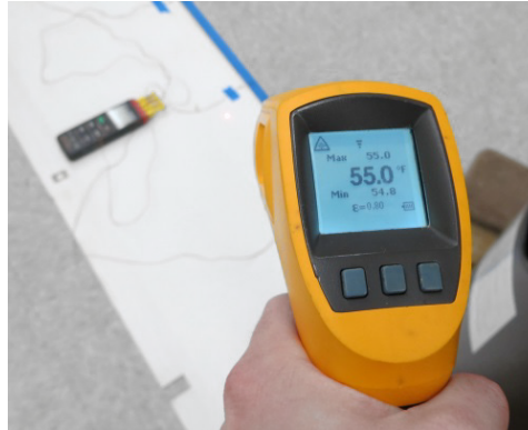
Figure 14: Measuring ambient temperature of plastic sheet
