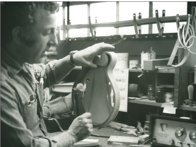
The tap tuning process is again brought back to Gibson’s old building. Peterson model 400 strobetuner at right.
