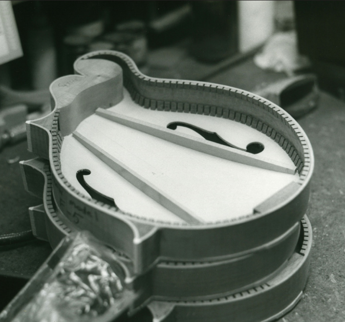
Three partially assembled bodies, with oversize tone bars, await the tap-tuning phase.
