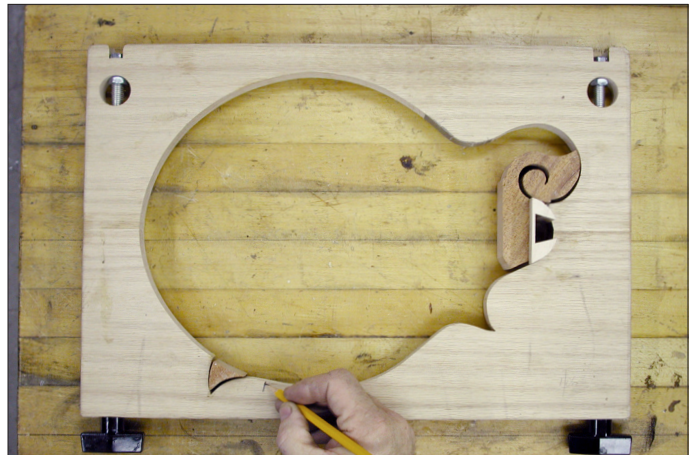
2. Position lower point block in fixture and make a mark on the fixture where the long rib piece will end.
