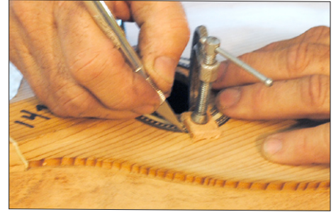
3. Use a sharp #11 X-Acto blade and score a line into the soundboard on the inside and outside of the rosette.
