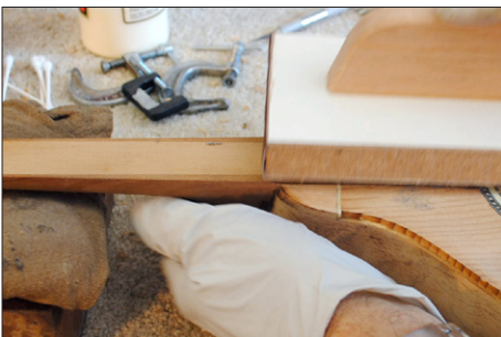
25. Ensure that the sanding block is square to the fretboard plane so that it does not alter the shape of the fretboard plane.
