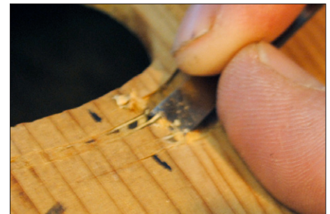
9. Wiggling the gouge back and forth may be helpful in working the tool through the wood.
