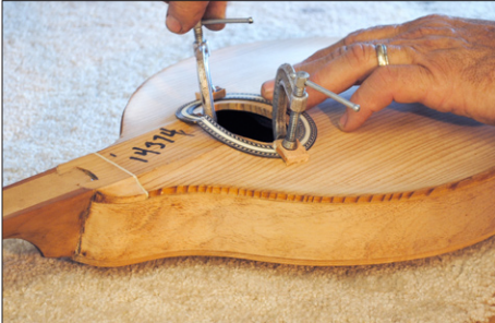
4. Place two more cauls and clamps on the rosette, then remove the first two clamps, and complete the cut.
