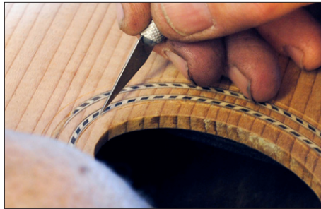
5. Remove the rosette and deepen the cut you have made. The depth should equal the rosette's thickness.
