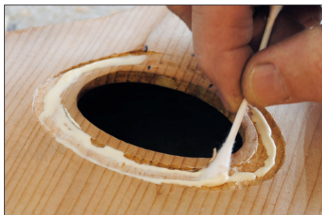
14. Use a Q-Tip to spread the Titebond evenly into the channel.
