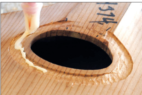
13. After you confirm the depth of the channel, apply a thin bead of Titebond Regular Glue into the channel.
