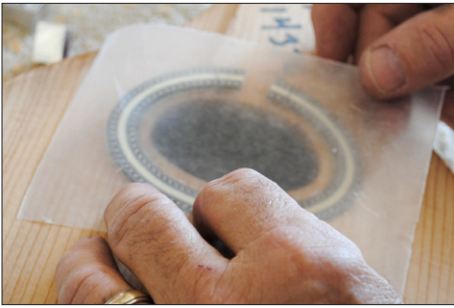
16. Use wax paper to prevent cauls from being glued. Use a big piece and cut through it or use several small pieces.
