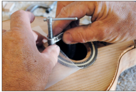
17. Place wood cauls on the wax paper and begin to position small C-clamps around the rosette.
