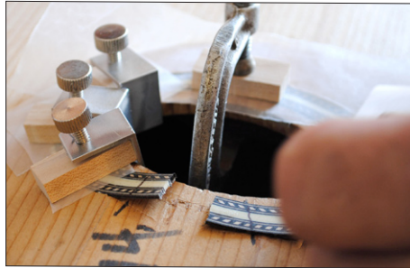
20. The split part of the rosette will bend upwards. It gets the last clamp (Fig. 22).
