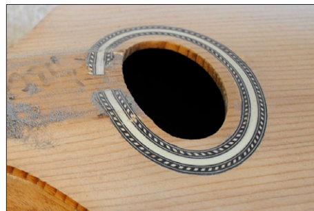
26. Sand the open ends of the rosette flush to the fretboard plane.
