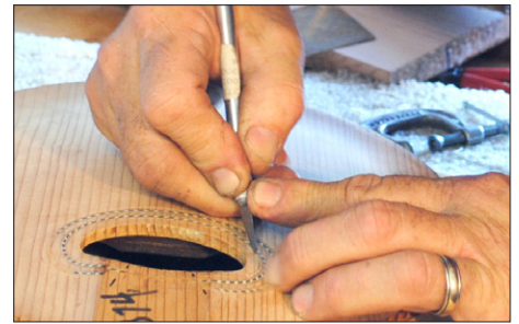
6. Be careful that you do not chip out the soundboard wood when working near the soundhole's edge.
