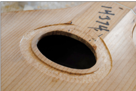
10. Work the channel up to the fretboard plane, but do not attempt to cut the channel level to the fretboard plane.
