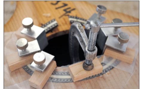
21. Snug all the clamps evenly and ensure that the rosette is properly seated in the channel.
