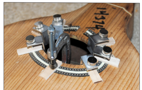
12. Using small clamps and cauls, test-clamp the rosette. Do not clamp the ends of the rosette down to the fretboard plane.
