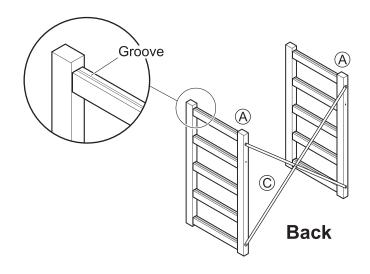
Refer to "Inserting Shelf Boards", and install (B) shelf boards starting from the bottom shelf. \* Install the shelf boards according to the height of items to be stored.
