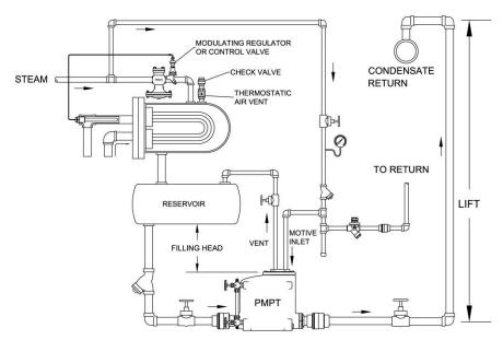
Figure 4: Closed Loop Pump System
