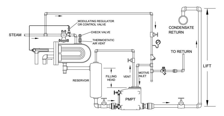
Figure 5: Closed Loop Pump System with Vertical Reservoir when Fill Head is Restricted
