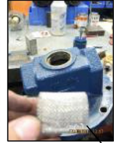
Remove, inspect and clean strainer.
