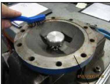
Clean gasket surfaces.
