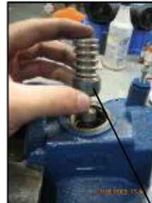
Remove spring & disc. Clean and lap disc to seat.
