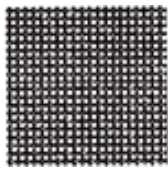
20 MESH Wire Dia. 0.015 Opening 0.034 49% Open Area
