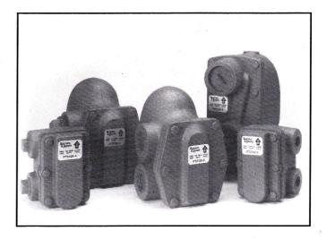
to be discharged. The float is designed to provide sufficient buoyancy to overcome the differential pressure across the valve. The internal float and valve configuration is such that the condensate level is always above the valve, creating a continuous water seal at the seat.
