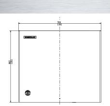
mm[inches] 908 [35-3/4] ELECTRICAL SUPPLY 7/8" DIA. OPENING 558 WIRE HARNESS CONNECTION 7/8" DIA. OPENING (SRK-10J ONLY) 90 211 186 [8-1/4] [7-3/8] 380 SUCTION LINE 5/8" FIELD CONNECTION
