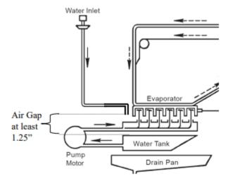
In all of our ice maker models, the built in air gap described above are secondary back up to the water
