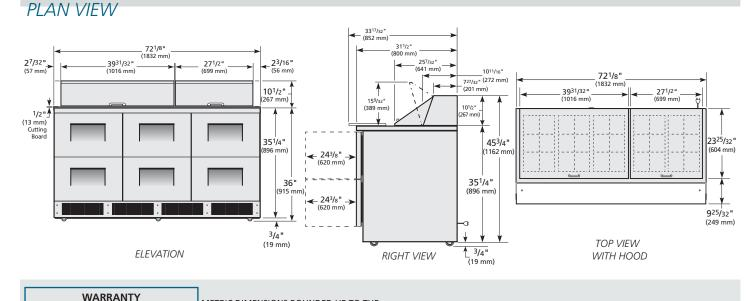
METRIC DIMENSIONS ROUNDED UP TO THE Three year warranty on all parts NEAREST WHOLE MILLIMETER and labor and an additional 2 year warranty on compressor. (U.S.A. only)
