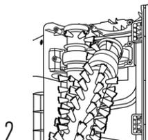
2 With belt in place, pull and slide brush roll into unit, making sure that the brush roll end caps are in correct orientation.
