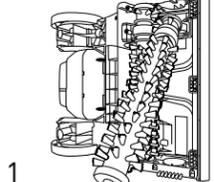
1 Slip brush roll through belt. Make sure belt is centered on pulley when replacing.
