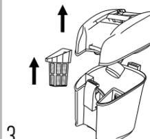
3 Unlatch the lid to remove the top. Remove the filter basket and clear any debris. Empty the tank, rinse, and allow to air dry.
