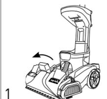
1 Remove the nozzle cover by pulling up and forward on the latch.
