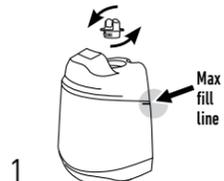
1 Lift up to remove the Clean Water Tank, then remove the cap and add warm water to the fill line. Add 3oz. of Hoover Solution. Secure cap.
