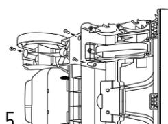
5 To remove belt, unscrew foot side cover from underside (3 screws).
