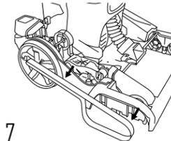
7 Slide belt off shaft and remove. If replacing belt, install the new belt.
