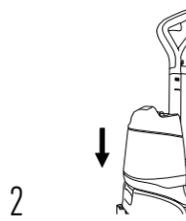
2 Align the tank and firmly press it into place.
