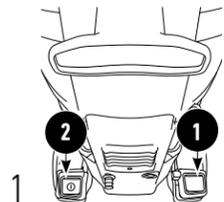
1 Step on the Handle Release Pedal to recline the cleaner for cleaning position.
