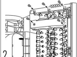
2 Lay the product down to access the underside. Use a Philips screwdriver to remove 6 screws. Arrows show location of screws on the underside of your cleaner.
