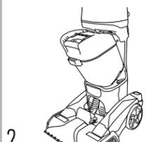
2 Grab the Dirty Water Tank handle and pull up to remove.
