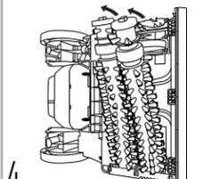
4 Pull both brush rolls out toward user to remove from cleaner. Belt will still be attached to cleaner.
