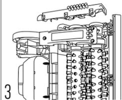
3 Remove underside belt cover and the brush roll end cap.
