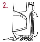
Wrap the power cord around the cord hooks for convenient storage.
