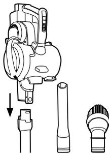
1 Press the handheld release button. Pull to separate the handheld from the reach wand.
