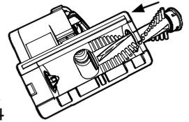
4 Re-fit the brush roll into the housing and turn the brush roll lock clockwise to lock.
