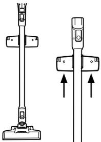
1 Choose the desired location, then place the mount on the wall at the desired height. Mark the wall anchor locations. Install the anchors and screw the mount to the wall.
