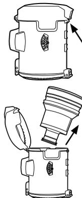
1 Pull open the lid of the dirt cup to access the filter. To clean the cyclone, lift to remove. Clean dirt and debris.
