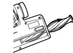
2 Pull the brush roll out of the powered nozzle. To remove any threads or hair, slide the blade of a pair of scissors into the groove of the brush roll and cut along the groove.
