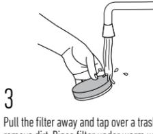
3 Pull the filter away and tap over a wash can to remove dirt. Rinse filter under warm water until water comes out clear. Allow filter to air dry for at least 24 hours until fully dry.
