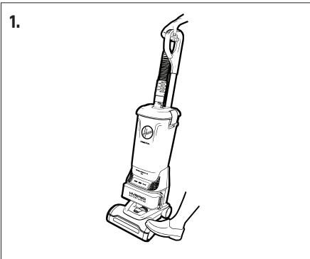
1. Place a foot where the foot icon is on the nozzle, then pull the handle back to recline.
