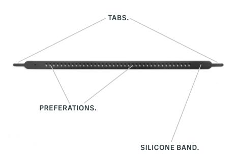
To lock the orthosis, the ends are overlapped and metallic tabs are secured through perforations.
