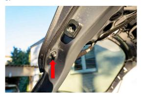
Also loosen and take off the 10mm Hex Nut on the left and right side.  $\,$
