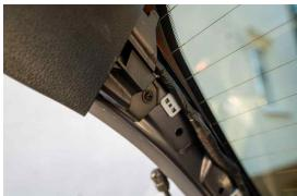
Loosen the phillips screw on both sides of the main cover part.
