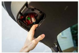
Now loosen and take of the main cover part by pulling or using the pry tool.
