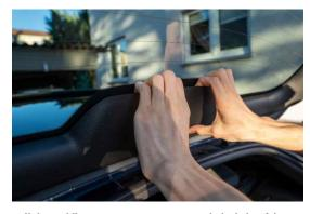
Pull the middle cover part or remove it with the help of the pry tool.
