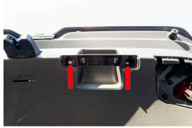
Remove the 3 service corvers. Remove the two 10mm Hex screws
