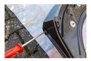
Insert a pry tool or a slotted screwdriver in between the trunk attatchment and the original spoiler to loosen it.
