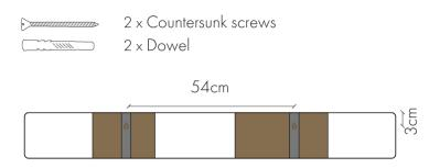
1. Mark the drill holes at the specified distances on the desired wall.
