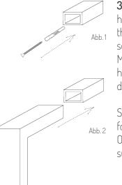
3. Insert the dowel into the hole and screw the socket to the wall with the countersunk screws. ( Abb. 1) Make sure that the pre-drilled holes for fixing NALI point downwards.
