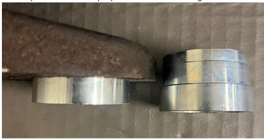
3. Press upper assembly in from top of C in the same manner as the lower assembly outlined in the previous step. (NOTE: the upper cup has a shorter shoulder.)
