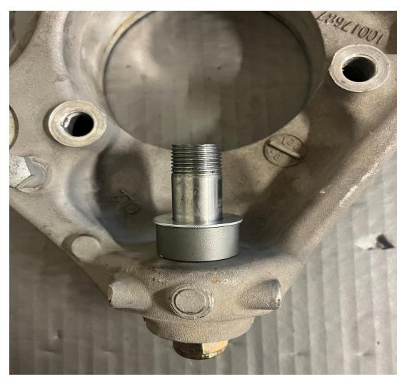
6. Grease the underside of the lower bearing and the top side of the upper bearing prior to sliding the outer knuckle studs into the bearings. This does not lubricate the bearing itself, it only impedes water/debris intrusion, bearings are pre-lubricated upon assembly. After sliding the studs through each assembly you should see the threads through the tops of each as pictured below:
