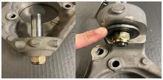
Prior to installing upper stud, insert the stock caster/camber bushing if it's not already in the outer knuckle. See pic above for reference. Using the hex pockets on the top of each stud, **TORQUE BOTH 9/16" NUTS TO 40 FT/LBS TO SEAT TAPERS.**
