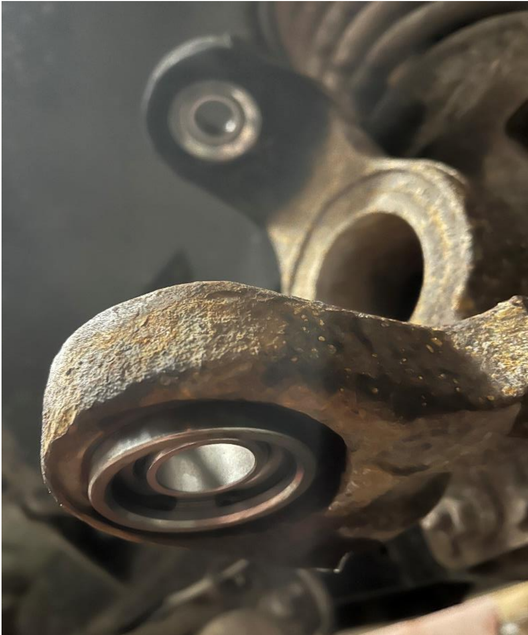
Figure 2: fully seated cups
