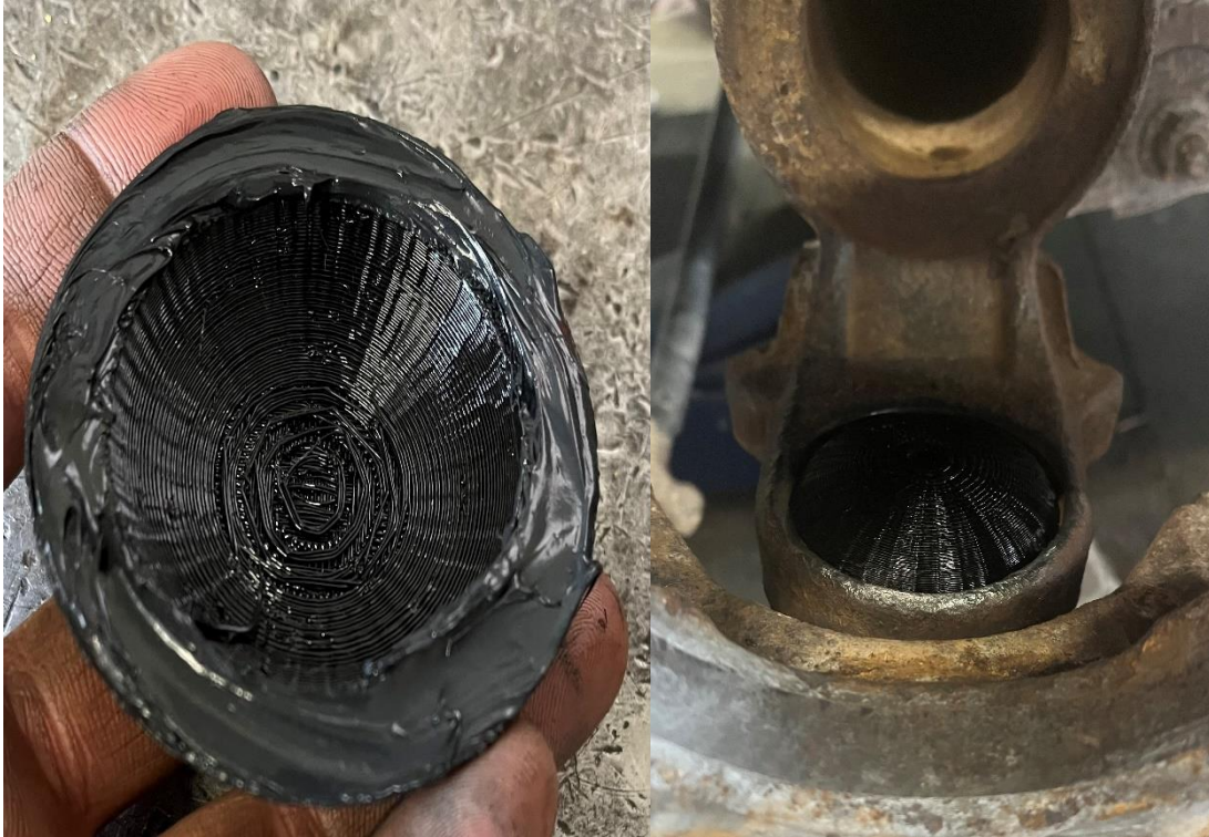
Figure 4: Dust cap installation
