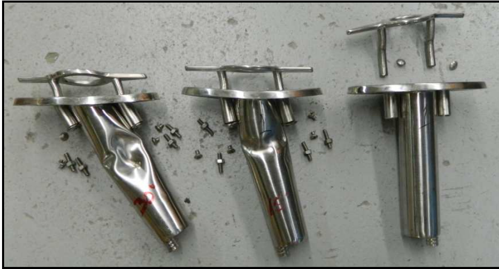
Views of the typical cleat samples following the tests.
