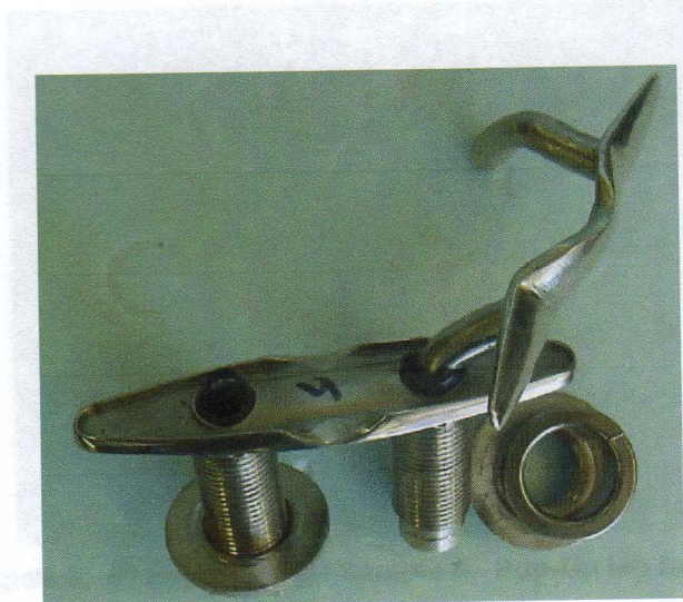
Figure 4. 4" Pop-Up Cleat Sample 4. Pop-up leg failure.
