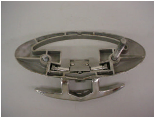
Figure 2. 6" Folding Cleat; typical failure mode (mounting bolt failure).
