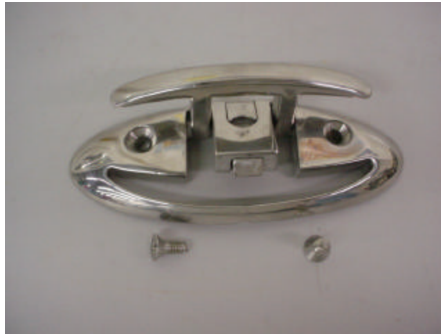
Figure 1. 4 1/2" Folding Cleat; typical failure mode (mounting bolt failure).
