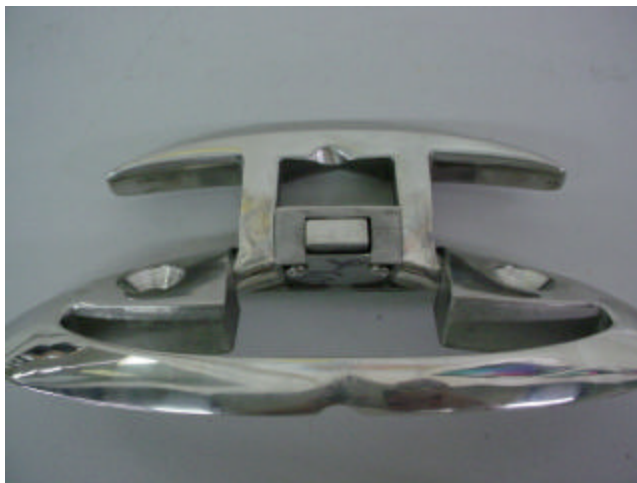
Figure 3. typical deformation experienced during tests
