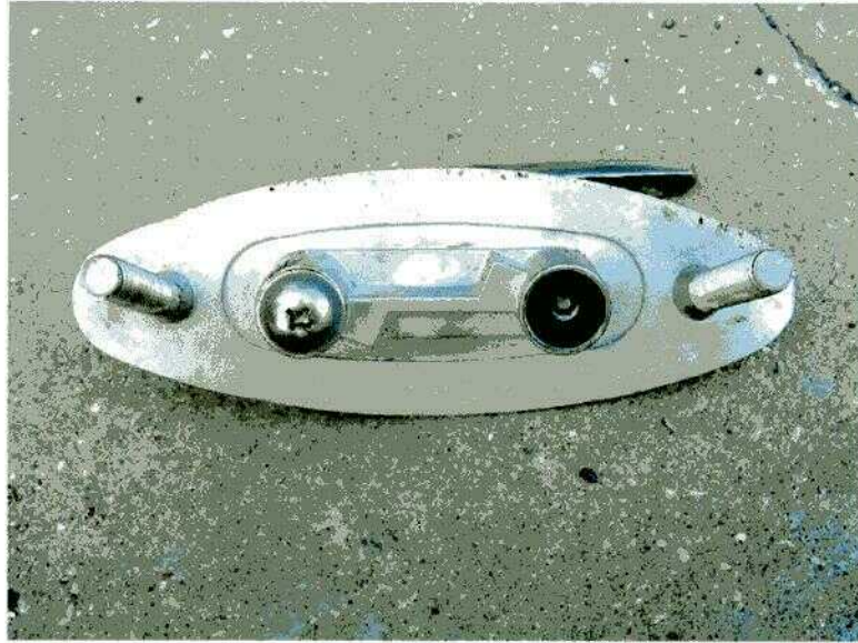
Figure 1. Wide-Line cleat; Typical failure mode (screw head failure).
