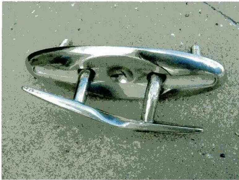
Figure 2. Wide-Line Cleat; Typical deformity.
