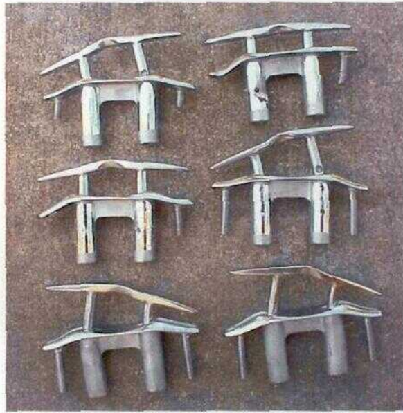
Figure 1. Photo showing Slimline Cleats after Pull Testing,
