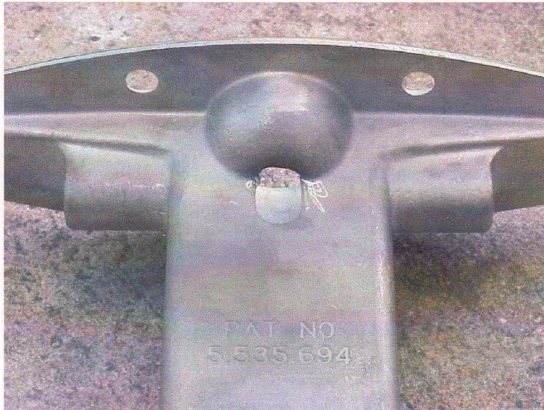
Figure 1. Photo showing typical “absence” of retaining pin due to vertical pull failure in 6 inch cleat.
