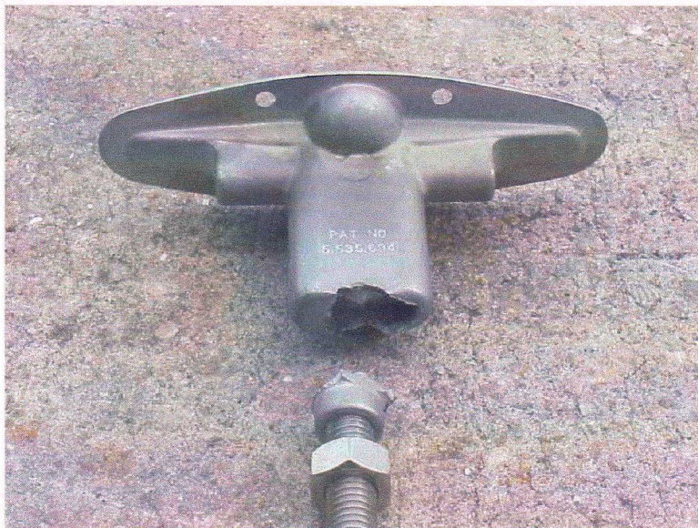
Figure 2. Photo showing typical Cleat Case Failure and remaining part left on threaded bolt. Note at top center of the 4 ½ inch cleat the first indications that the retaining pin is about to fail (small circle in metal).
