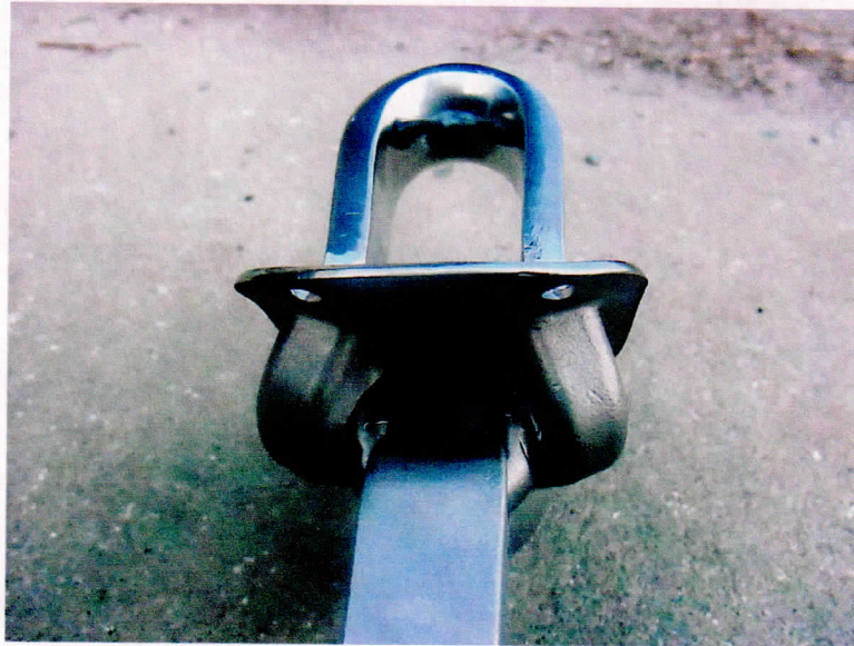
Figure 1. Oval Lifting Eye; Typical Failure Mode
