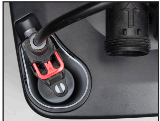
Brine valve and brine well system
