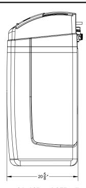
The Water Specialist – CWS-35 Cabinet accepts 35" tall mineral tanks up to a 12" diameter to maximize system capability.
