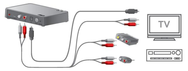
We recommend to connect **either** the TOSLINK input **or** the RCA input of the transmitter.
