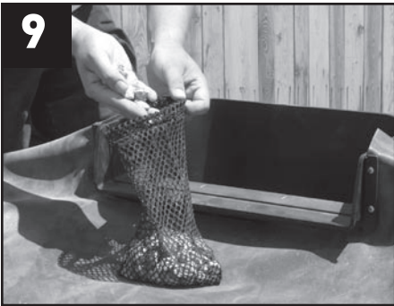
Fill the mesh bag with rocks for ballast. Use large gravel, lava rock or small stones.
