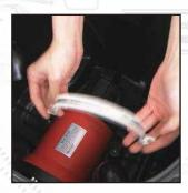
8. Take out the outlet pipe of the pump counterclockwise.
