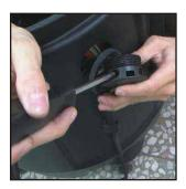
5. Use a 8mm Hexagon Socket Wrench to loosen a nut(part no.96) above of fixer (part no.97) and acorn nut(part no.95).
