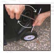
8. Toward the wire clamp thread to bucket and fix the pump wire in place.
