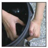
4. Use a long stick(like a 8mm Hexagon Socket Wrench) to lock both side of the outlet connector base convex (part no.114). Loosen the outlet connector base counterclockwise.
