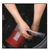
7. Remove the wire of the pump from the hole then take out the pump.
