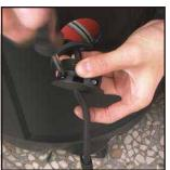
Fit the pump head with bucket and tighten a clip(part no.74).
